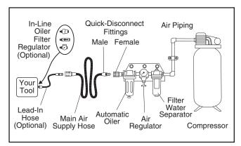
**Figure 5**. Recommended air supply system setup.
